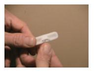
**Step 2)** Insert stake into hole in T handle, place on firm surface and tap with a rubber mallet until seated.
