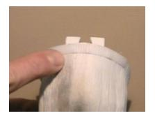
**Step 4)** Place a strip of **hook** side of "hook and loop" fastener around the rim of the base of the top of the feeder head.
